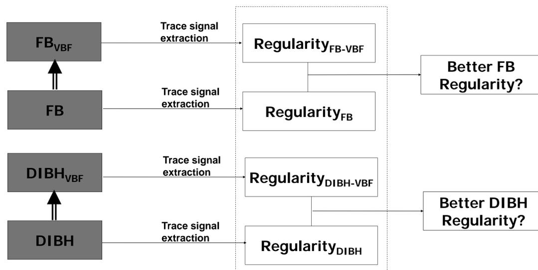
Fig. 1. The experiment setup and the trace signal processing diagram of the comparison between the regularity with and without the visual biofeedback (VBF). Shaded boxes indicate signal acquired and white boxes indicate the derived data.
