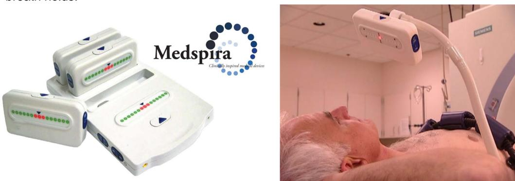
Fig. 2. Examples of the novel air-bellows belt system, the Medspira Breathhold, which features a compact and mobile LED based visual biofeedback (VBF) system to improve the regularity of patient respiration. Left: respiratory signal acquisition system; Right: the compact LED VBF.
